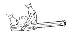
Chain brake unlock When the lever is fully pulled toward the operator, brake is unlocked.
